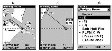
Route creation sequence, continued: Fig. 4. Point (3) set at channel mouth. Fig. 5. Fourth waypoint set further south along the beach, at a recognizable landmark (Bob Hall Pier). Waypoint PLFM Q W ends the route at an oil platform some distance from the shore. Fig. 6. Press **EXIT** to save the route and you return to this screen.
